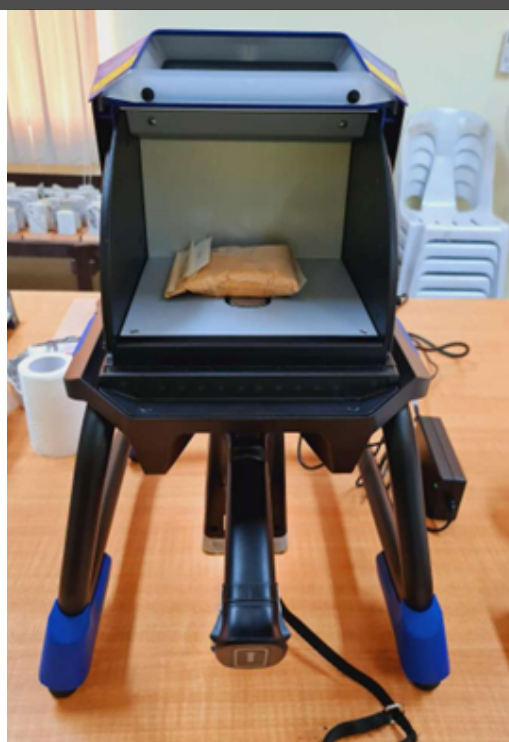
Using the pXRF to analyse drill cores (left), directly on top of pulps (middle), and using the workstation setup (right).
