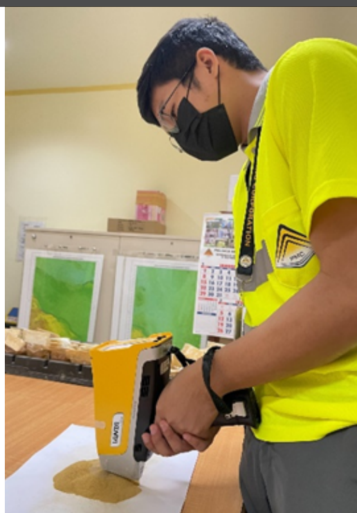
Using the pXRF to analyse drill cores (left), directly on top of pulps (middle), and using the workstation setup (right).
